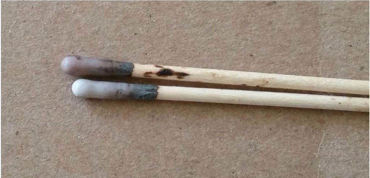
Defense Centers for Public Health – Aberdeen (formerly APHC), EHSD photo Figure B-2. Used Stick with Stain Next to Stick with No Stain
