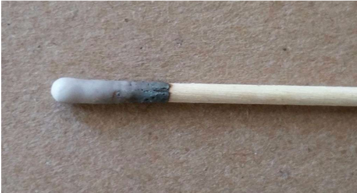
Defense Centers for Public Health – Aberdeen (formerly APHC), EHSD photo Figure B-1. Used Stick Tip with No Residual Fluid Stain
